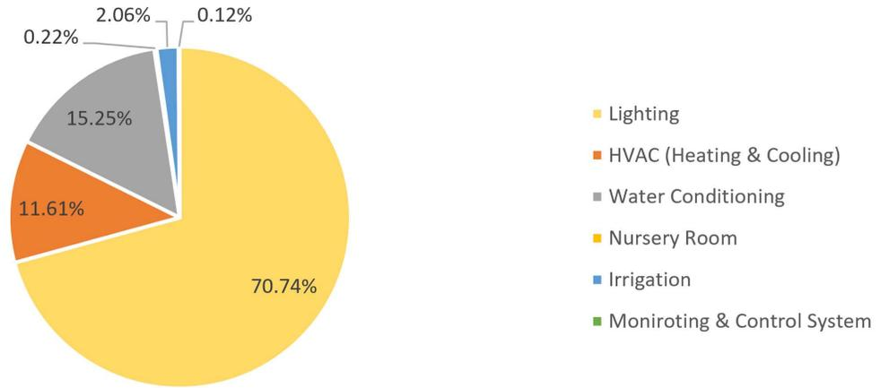
**Figure 1. Energy consumption breakdown per module for kale production**
